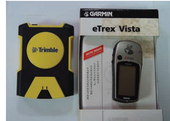
Fig 3-3-7 Satellite positioning device (left: device currently used)
