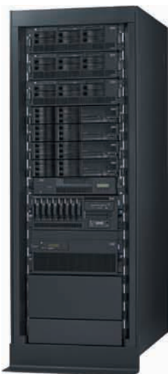
Fig 5-6 Rack-mount servers installed in a server rack
