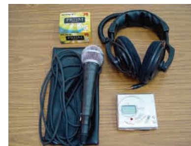
Fig 3-5-3 Audio recording equipment, from the left is mini-discs, professional earphones, professional microphone, and portable mini-disc recorder.
