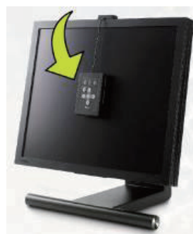
Fig.4-10 The controller is simply placed in front of the monitor for calibration.®
