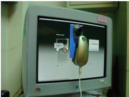
Figure 3. Using a spectrophotometer for monitor color calibration
