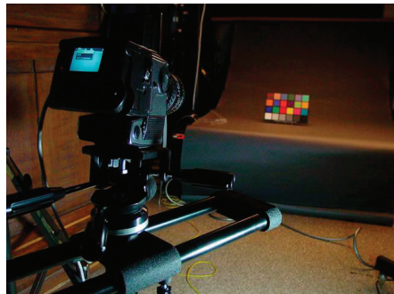
Figure 4. Conducting digital camera color calibration under a stable light source
